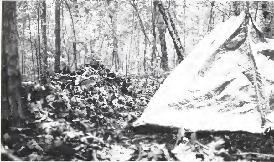
Figure 2 —Fuel buildup next to deployed shelter would generate considerable heat in an actual fire situation.
